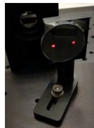
Figure 21: Both halves of a TiSapphire LASER beam visible on the Focusing Mirror.
