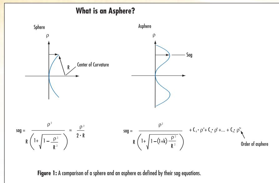
Figure 1: A comparison of a sphere and an asphere as defined by their sag equations.
