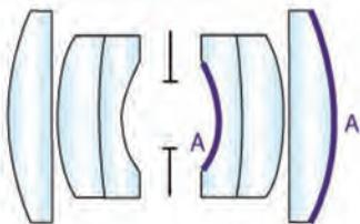
Figure 4: Conventional wisdom: asphere close to aperture stop and another close to image plane<sup>2</sup>
