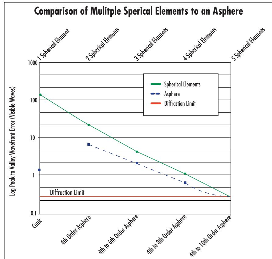
Figure 2. Wavefront error comparison for a multi element spherical system to a multi order aspheric polynomial. The aspheric element has one spherical side.
