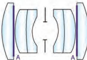
Figure 3: Asphere buried in system but symmetric about the aperture stop<sup>1</sup>
