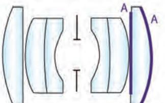
Figure 6: Dual aspheres on a single aperture stop in the aft optics<sup>4</sup>
